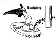
MOWING – Your trimmer is ideal for mowing in places conventional lawn mowers cannot reach. In the mowing position, keep the line parallel to the ground. Avoid pressing the head into the ground as this can scalp the ground and damage the tool.
